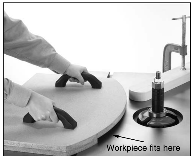
Figure 42. Pattern jig for making curved pieces.
